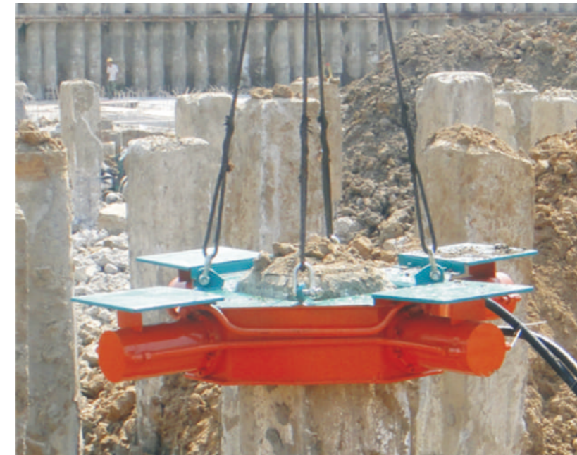
方型桩桩机的型号及参数: Hydraulic Square Pile Breaker Model and Parameters
