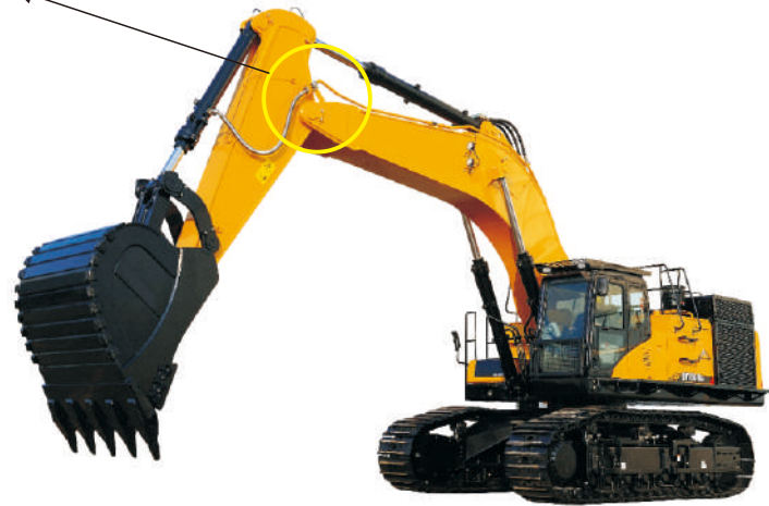
液压油管分离和安装部分 Hydraulic pipe separation and installation part
