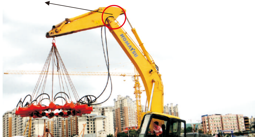
液压油管安装完成 Hydraulic pipe installation is complete
