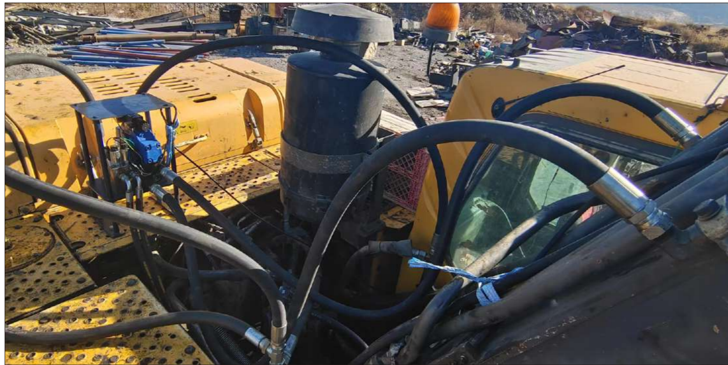
大阀固定焊接在驾驶室后面 The large valve is fixed and welded behind the cab.
