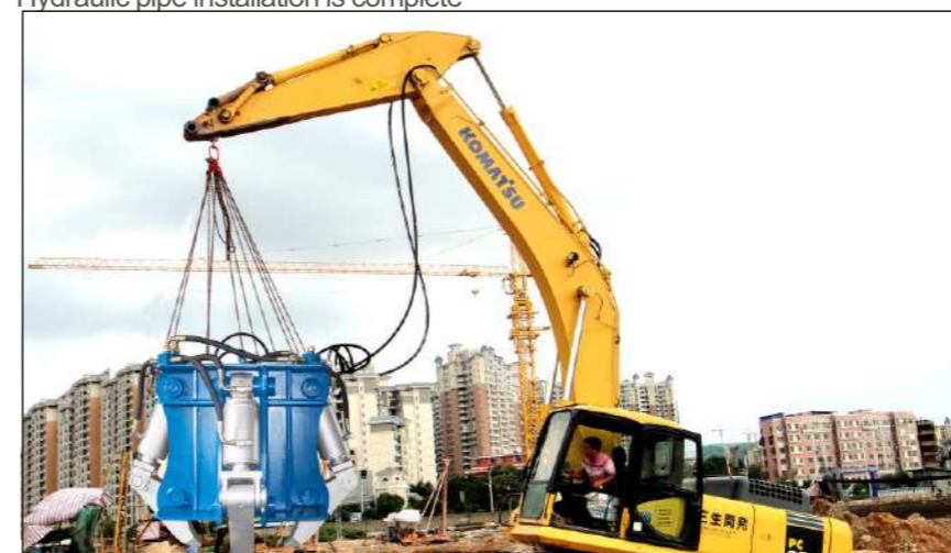
液压油管安装完成 Hydraulic pipe installation is complete
